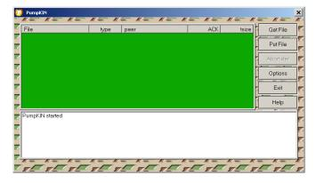
Click on Put File and Local file to be downloaded (Modbus\_TCP). Enter password G5 (case sensitive, must be upper case G) in Remote file. For Remote host, enter the IP address of the Micro PLC (for example: 10.10.0.2).
